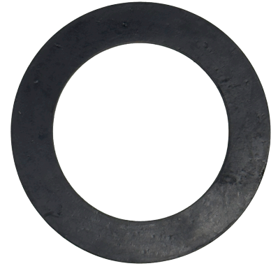
Flush Valve Gasket O.D.: 3-1/8" I.D.: 2-3/16" For Style 210
