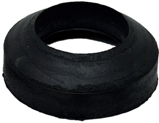
Tank to Bowl Seal with Hex With Recessed Hex OD: 3-1/2" ID: 2"
