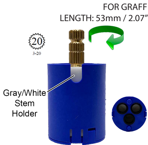
DIAMETER: 28mm OEM # 5057650 / KEROX # KRJ-28 CLOSES COUNTER-CLOCKWISE CC19114
