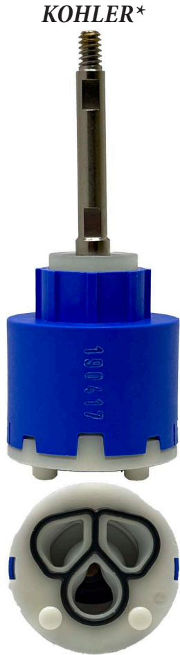
Ceramic Cartridge CC19156 3.37" 10-24 Thread OEM: 1090948
