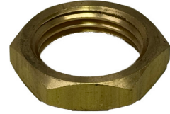
Brass Faucet Shank Locknut AB11888 1/2-14 NPS
