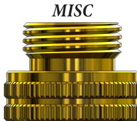
MISC Hose Bib Adapter 145380 .938" 1-1/16-20 x 3/4-11.5 GHT 1-1/4" Hex. Includes O-Ring.
