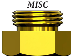
MISC Hose Bib Adapter 130080 .938" 1-1/16-20 x 3/4-11.5 GHT Nickel Plated. Includes O-Ring.
