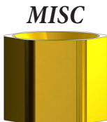
MISC 9/16-20 X 3/8-18 NPS (21/32- 18) Female Adapter 146200 .605"
