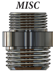
MISC Adapter 154040 .610" 3/8-18 NPS X 3/4-11.5 GHT Adapter
