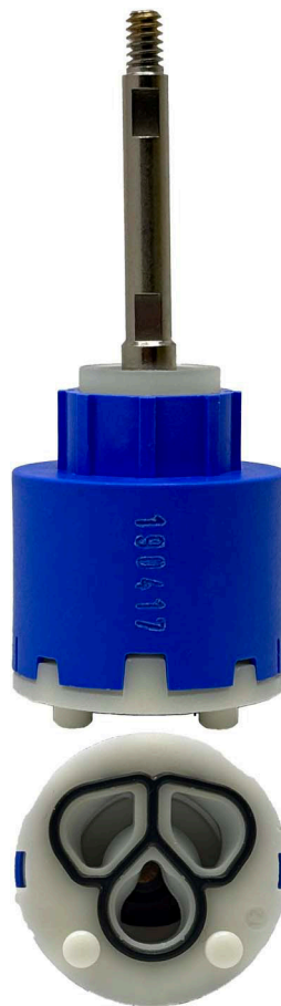
Ceramic Cartridge CC19156 3.37" 10-24 Thread OEM: 1090948
