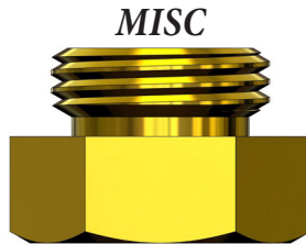
Hose Bib Adapter 145380 .938" 1-1/16-20 x 3/4-11.5 GHT 1-1/4" Hex. Includes O-Ring.
