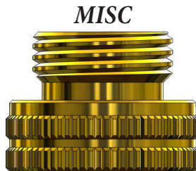
Hose Bib Adapter 146040 1.050" 1"-11.5 NPS x 3/4-11.5 GHT
