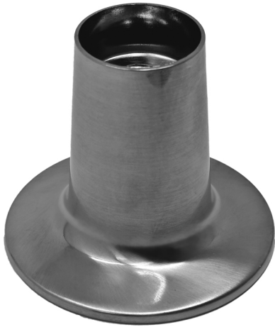
Chrome Plated Escutcheon PP50401-BN 2-3/4" O.D. X 2-1/4" High X 21/32-18 Thread Brushed Nickel
