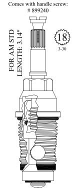
$\begin{array}{c} \text{gasket: 890170 o-ring included} \\ 430022 \end{array}$
